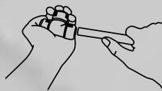
Hole the fitting horizontally to the pipe and push the pipe firmly into the fitting. The connection is complete when the socket of the fitting has reached the next ^ mark on the pipe. Do not undo the retaining cap.
