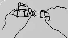
Unscrew the retaining cap from the fitting and pull out the pipe.
