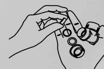
Reassemble the fitting by inserting a new grab ring together with the spacer washer and O' ring. See illustration overleaf for the correct order for reassembly. Hands tighten the retaining cap. Check the end of the pipe for damage and re-cut if necessary.
