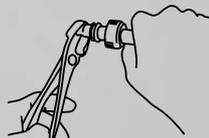
Use pliers to flatten the teeth on the grab ring and remove. The spacer washer, O' ring and retaining cap can then be removed from the pipe.
